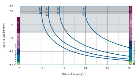
Natural frequency of a single-degree-offreedom system consisting of a fixed mass and an elastic bearing consisting of VIKAFOAM VF 1300 on a stiff subgrade.
